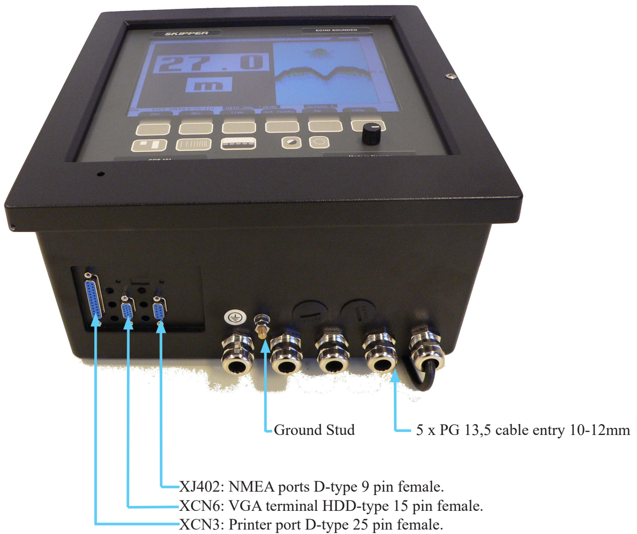
Fig. 3.5. Data Communication Interfaces.
